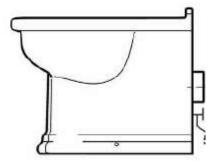
Wall hung: the toilet pan is bolted to a metal frame within a wall or boxing, with the cistern being hidden within the framework behind the pan.
