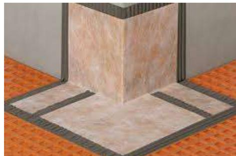
1. Fit the 'internal corner patch' first, wrapping it around the external corner.
