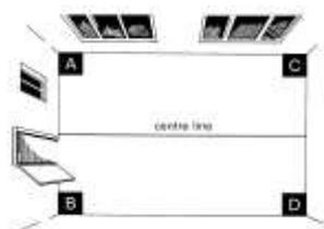
Step 2: Measure and divide your central line by two to split it in the middle, mark and repeat the process above to work out your cuts in the opposite direction.
